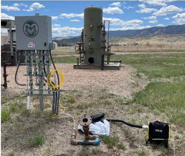
*Figure 3: High range quantification accuracy test setup at CSU's METEC facility. Gas is metered by the control box on the left and delivered to the expansion nozzle.*
